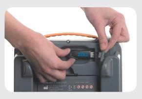
Plug a memory stick into the USB port to download rescue event data, upload a new configuration or upgrade software.
