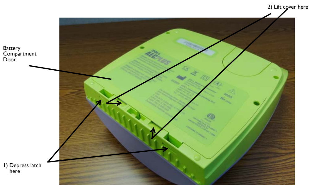
Figure 7: Removing the Battery Compartment Door
